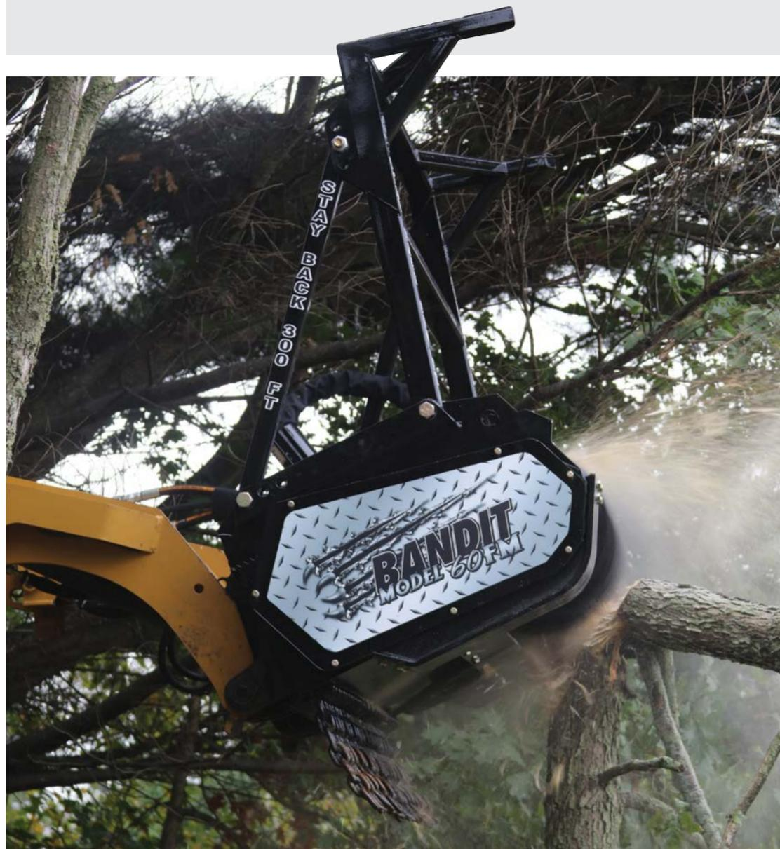
The **exclusive anvil** that is standard on every Bandit head acts as a second cutting surface, producing the best end product on the first pass. This **improves productivity** and **reduces fuel consumption**, while also preventing material from jamming the drum, a common problem among competitor's equipment.
