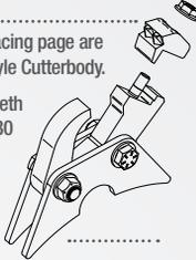
Fig. 1: Knife Style Cutterbody
